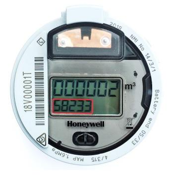
Top line displays billable units in cubic meters or kilolitres. Reading shown = 2 m<sup>3</sup> or 2 kl
