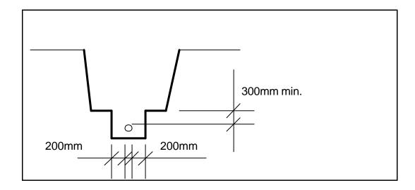
Where excavation exceeds the required depth by more than 200mm, the excavated material shall be replaced with stabilised sand or approved compacted fill to the required level.
