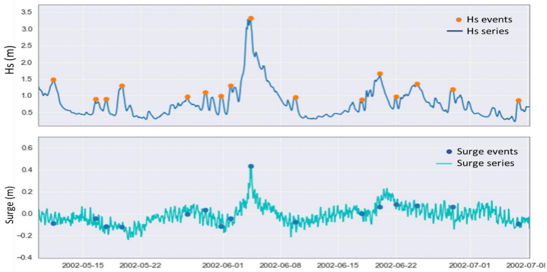
Figure 3-8: Declustering of discrete weather events in wave record (top), and corresponding surge record (bottom)
