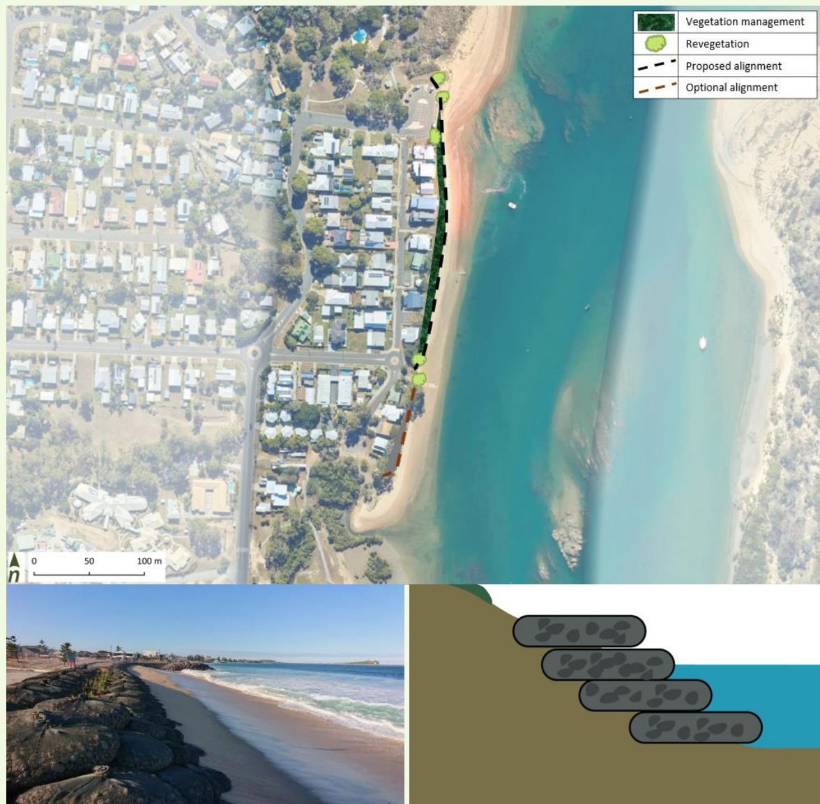
Figure 27. Island Esplanade foreshore – Option 4 – Concept plan of AquaRock bag revetment replacement. Photo (bottom right) sourced from Gabion Cages and Baskets 3 .
