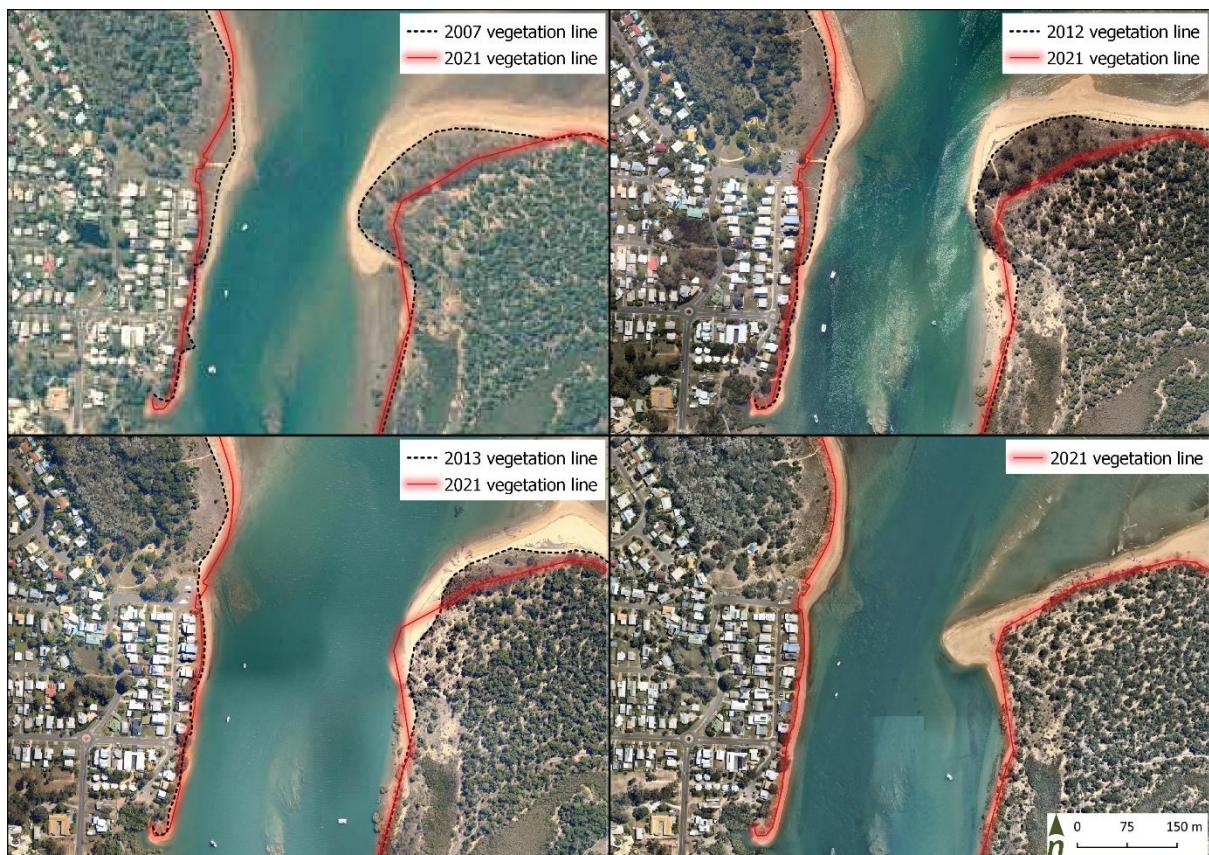
Figure 16. Historical aerial imagery for Island Esplanade with indicative 2007 to 2021 vegetation line.
