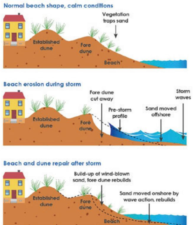
Figure 4. Natural short-term erosion and dune rebuilding process
