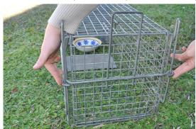
3. Pull horizontal bar up to top of cage. Trigger is hooked over handle and should look like this.
