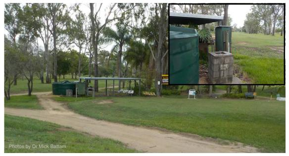
**Figure 5.1:** Due to its close proximity to the 9<sup>th</sup> tee, recycled water is likely to spray onto the adjacent roof that is harvesting rainwater or the adjacent drinking bubbler (insert). The irrigation system needs to be set up so this does not occur.
