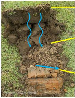
**A1 horizon:** 200 mm of sandy loam that was moderately structured. This horizon had been removed in some areas, with gravel observed at the surface.
