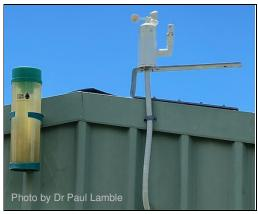
Figure 8.4: Weather sensors on the pump shed.
