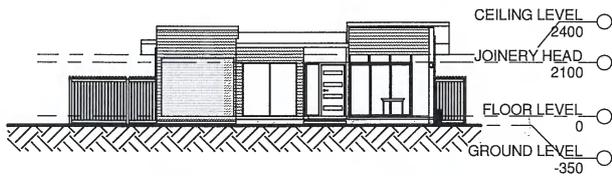
6 Unit Type 3 - Single Garage - Front Elevation
