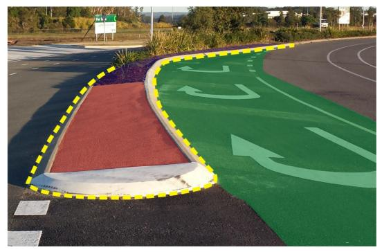
Figure 32 – Example of Road Edge Structure
