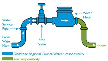
On the top of your water meter is a panel containing a series of digits. The black digits represent the kilolitres of water passing through your meter.
