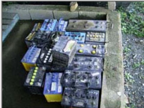
Australia produces approximately 3.8 million spent lead-acid batteries per year. The plastic, lead and sulphuric acid used in batteries are all recyclable, however the correct storage and disposal of batteries is important to ensure protection of both the environment and the health of the community. Incorrectly stored batteries have the potential to release sulphuric acid and lead into the surrounding environment and contaminate soil, stormwater and water ways. Lead is a highly toxic sub-
